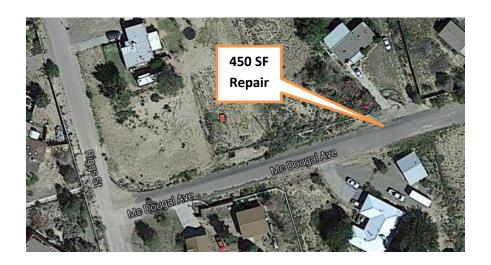
Assessment: Significant surface, base and roadway edge deterioration
